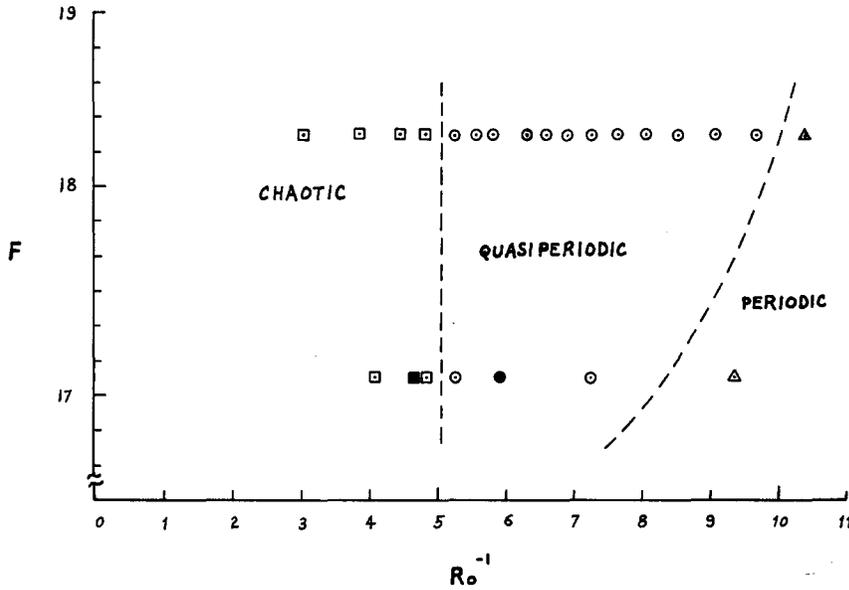
Fig. 1. Summary of experiments. The experiments at parameter values marked in black are presented in detail in figs. 2 and 3.  $F = 4\Omega^2 L^2 \rho / (gH\Delta\rho)$  is the Froude number, and  $R_0 = \omega/2\Omega$  is the Rossby number.
