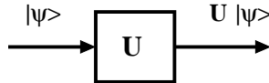
FIGURE 8. The diagram representing the action of a unitary matrix U corresponding to a quantum gate on a qubit in a state |\psi\rangle .
